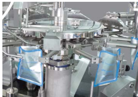
Pouch Opening & Filling - With a certain pouch opening with vacuum cups and mechanically gripping the pouch, the product will be positively filled into the pouch.
