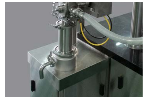
Liquid Filling Pump - The pump is installed out of the frame making the cleaning easy.
